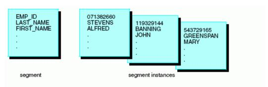
The relationship of a segment to its instances is illustrated in the following diagram.
