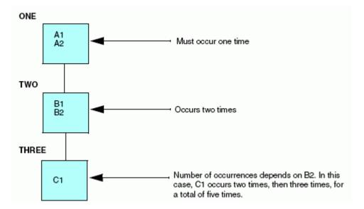
Since field C1 repeats with relation to fields B1 and B2, which repeat in relation to fields A1 and A2, field C1 is described as a separate, descendant segment of Segment TWO, which is in turn a descendant of Segment ONE.
